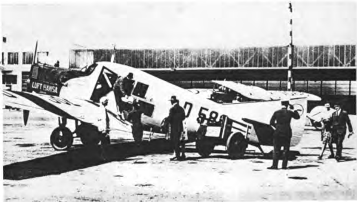
The world's first strut-free all-metal low-wing monoplane with a closed cabin, the Junkers F 13, was one of the great commercial aircraft in aviation history. It was designed and built in six months and entered service in Germany in July 1919. Carrying four or five passengers in a comfortable heated cabin, it was widely used for two decades. They operated as landplanes when equipped with wheels or skis, or floatplanes when fitted with pontoons. The last one in service was retired in Brazil in 1947.
